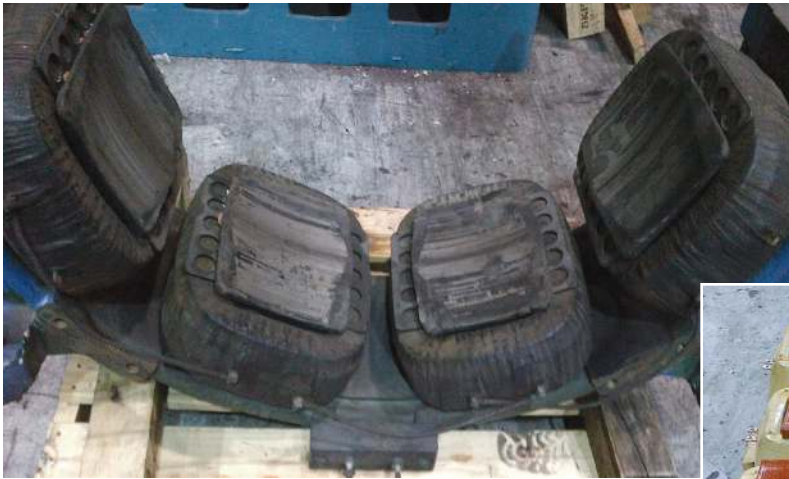
(l-r) Gearless field coils before refurbishment and after, installed on shoe coils
