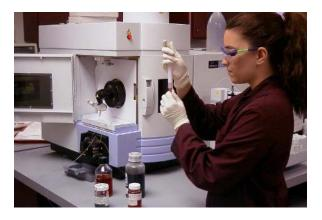
to the oil. These particles are so small that they remain suspended in the oil. Many products of the facilities process are also trapped in the circulating oil as well as internal contamination. Classifying and measuring this contamination reveal the rate of wear and level of contamination. Therefore, the oil becomes a working history of the machine. A good oil analysis also proposes methods to reduce accelerated wear and contamination.
