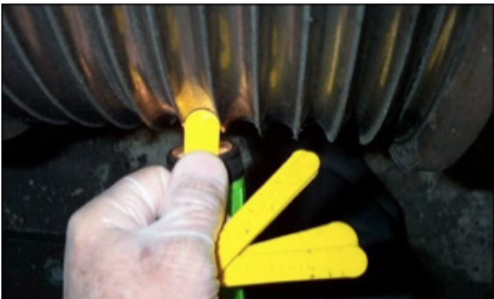
Grooves being checked with groove gauges
