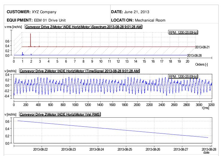
**DESCRIPTION:** Initial vibration readings collected on June 21, 2013 indicate possible structural looseness at the motor mounts. Follow up vibration readings were collected on June 23, 2013 while stiffening the motor mounts. Significant reduction in vibration amplitude recorded during this test.
