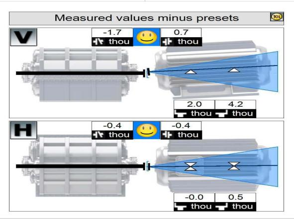
**DESCRIPTION:** Machine alignment corrected and machine is within tolerance.
