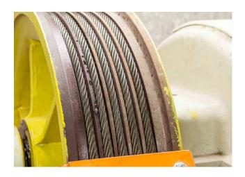
The U-groove sheave is largely seen in older elevator installations. It is the sheave of choice, delivering the best possible rope life. Its size is comparatively large to newer sheave styles, but this size in conjunction with strong grooves reduces wear to ropes, including fatigue and abrasion. Adversely, however, its wide diameter doesn't support today's traction needs.
