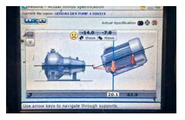
as they can work on high-resolution, non-contact technology and can measure down to 0.0001 mm. This form of alignment also eliminates the risk of reading errors that are typical of low-resolution readouts and sticking dial hands and provides consistent results regardless of the operator. Additionally, the laser systems can generate reports directly from the measurement instrumentation, allowing for faster delivery and analysis of the results.
